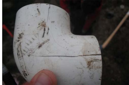
**Split PVC 90° Angle Caused by High Water Pressure**
